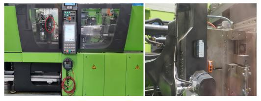
**Figure 1.** The left image shows an injection molding machine with a mounted 3-axis accelerometer (sensor marked by a red circle in the center of the image). The right picture shows the mounting of the same sensor in detail.
