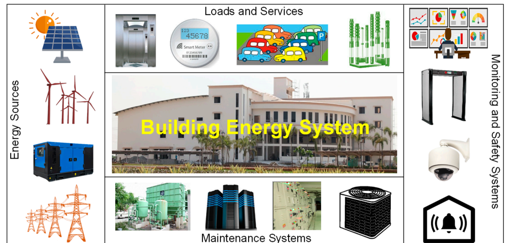
Figure 2. Constituents of a smart microgrid associated with a building.
