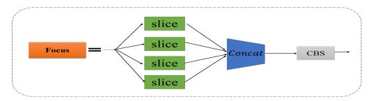
**Figure 2.** Focus network structure. The structure is mainly to slice the feature into four parts, and then perform the Concat in the channel dimension.
