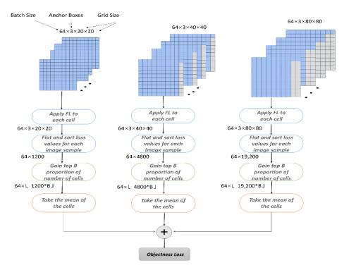
Figure 7. Comprehensive loss function calculation diagram.
