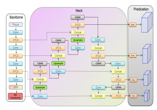
**Figure 3.** Network structure diagram of improved YOLOv5. The overall network structure consists of three parts: backbone network, feature fusion network and output layer.
