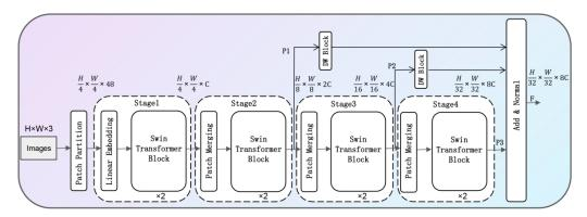
Figure 4. MS Transformer module structure.
