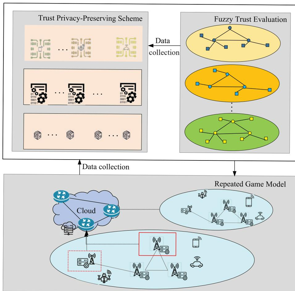
**Figure 1.** The framework of the fuzzy-based privacy-preserving scheme based on the repeated game. The devices in the solid line frame are common IoT devices in the cluster, and the dotted line is the routing device that guarantees data uploading.
