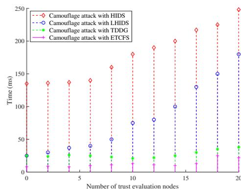
**Figure 6.** The time consumption with cluster formulation under different schemes in camouflage attack (hop limit = 2).
