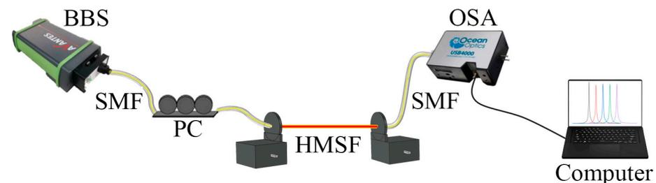
**Figure 2.** Schematic diagram of the experimental device.
