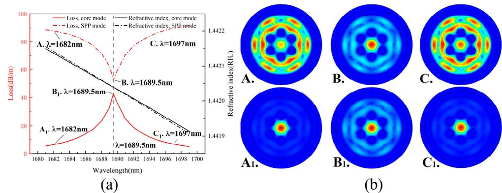
**Figure 6.** (a) Coupling relation diagram between the SPP mode and the fundamental mode; (b) schematic diagram of the mode field of SPP and fundamental modes in the coupled band.
