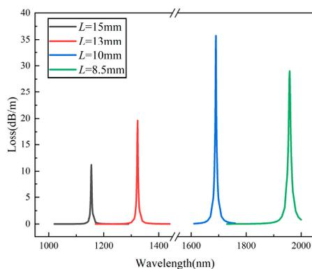
**Figure 5.** Confinement losses for different pitch  $L$ .
