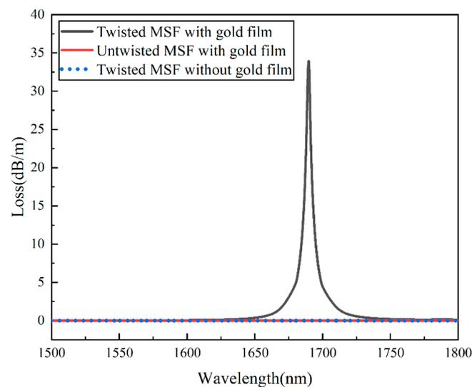
**Figure 3.** Comparison of the losses of HMSF with gold film, untwisted MSF with gold film, and HMSF without gold film.
