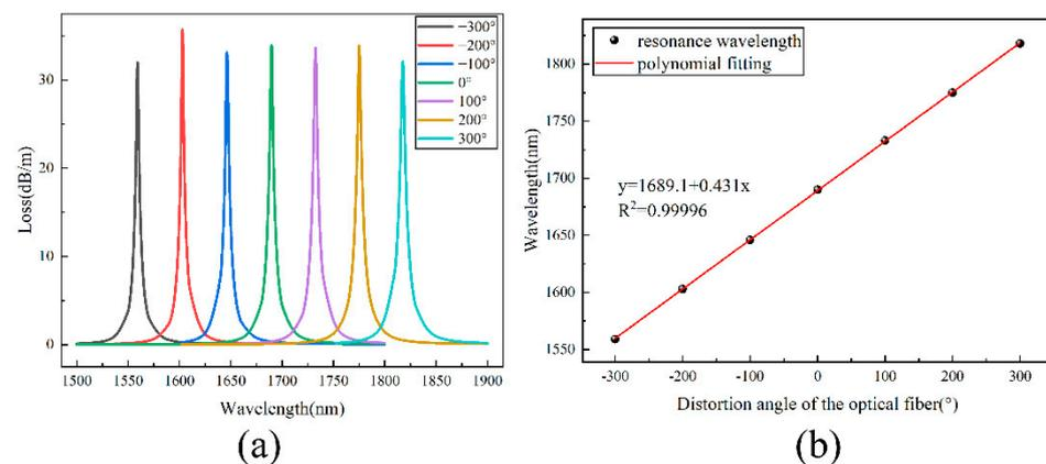
**Figure 7.** (a) Loss spectra of HMSF with different additional torpor; (b) fitting relation between the resonance wavelength and the additional torsion angle.
