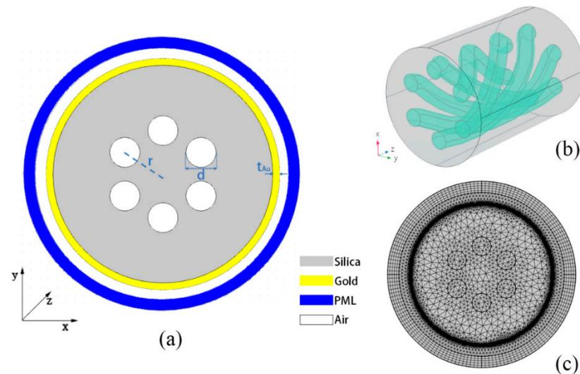
**Figure 1.** (a) Schematic diagram of the designed HMSF; (b) 3D structure diagram of the HMSF; (c) fiber diagram with a meshing grid.
