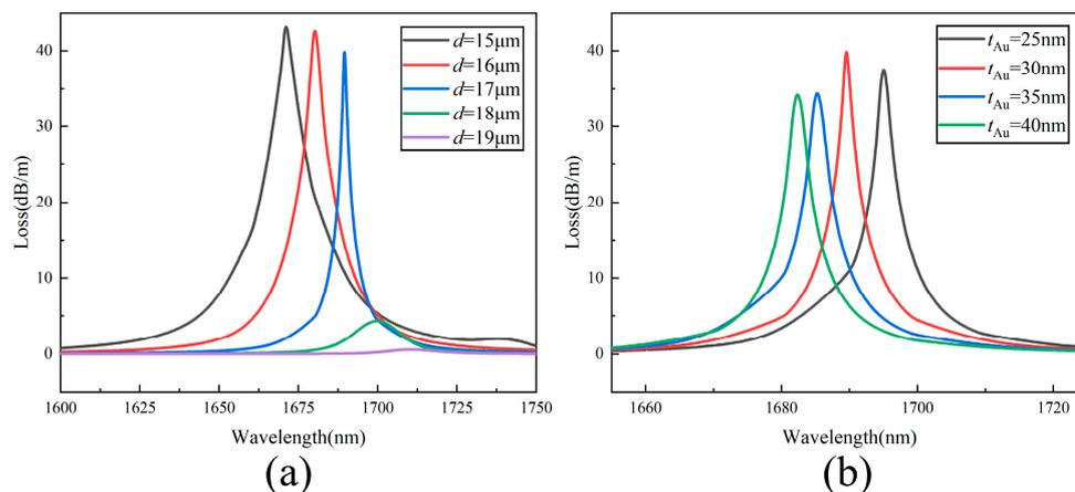
**Figure 4.** (a) Confinement losses for different air hole sizes  $d$ ; (b) confinement loss for different thicknesses of the gold film.
