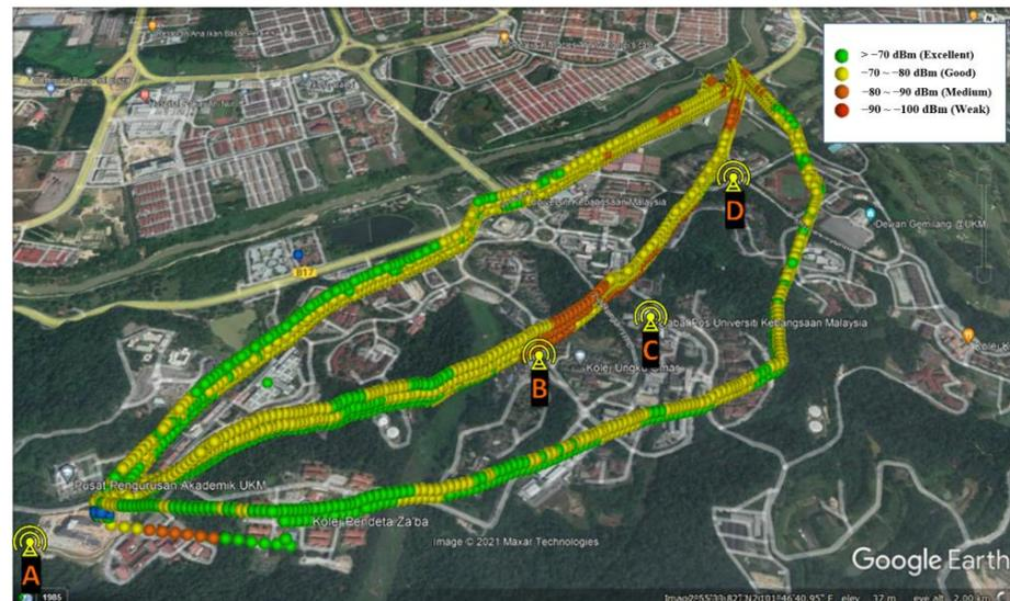
Figure 5. Measured RSRP values at different routes and elevations.
