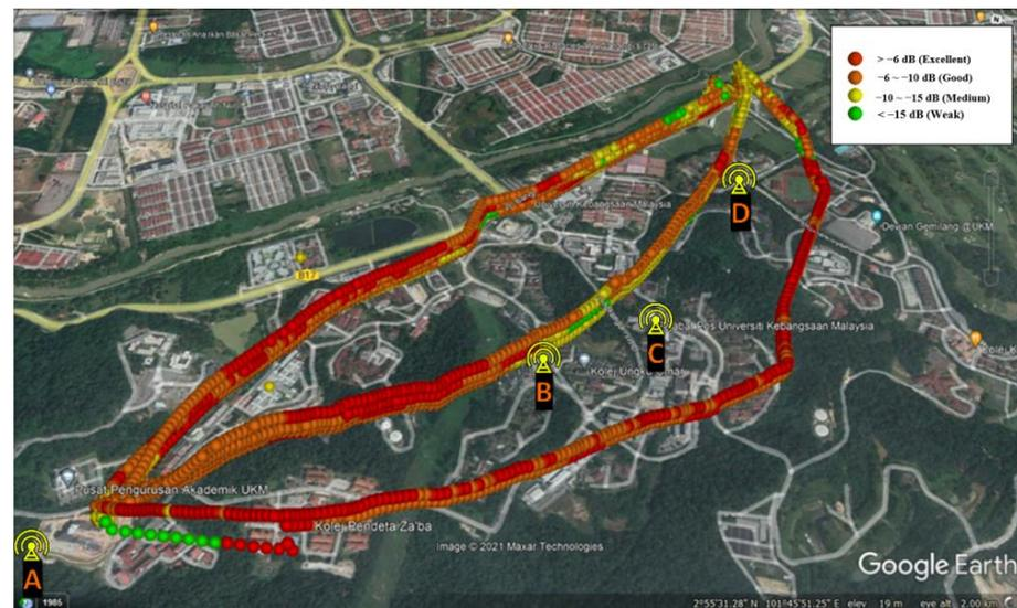
Figure 6. Measured RSRQ values at different routes and elevations.
