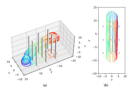
**Figure 6.** The visualization of the executed trajectories for large-scale UAVs formation flying through an obstacle-rich area. (a) Full view of the trajectories. (b) *xoy*-plane projection trajectories.
