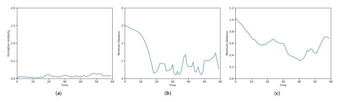
**Figure 7.** Illustration of the performance of interaction terms for MFG control ( $\mathcal{F}^1$ ,  $\mathcal{F}^2$ ,  $\mathcal{F}^3$ ). (a) Formation similarity error. (b) Minimum distance between UAVs and obstacles. (c) Minimum distance between UAVs.
