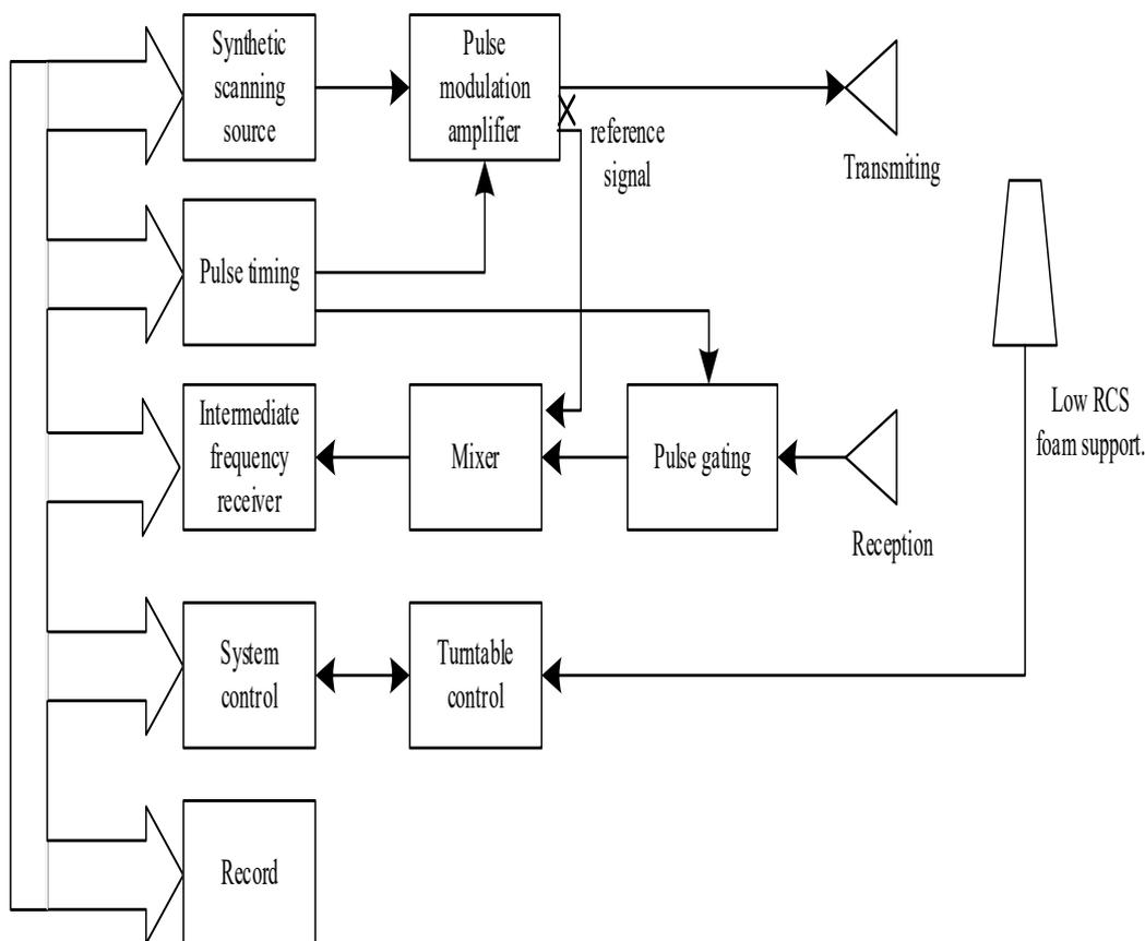
**Figure 1.** The block diagram of the RCS measurement system.
