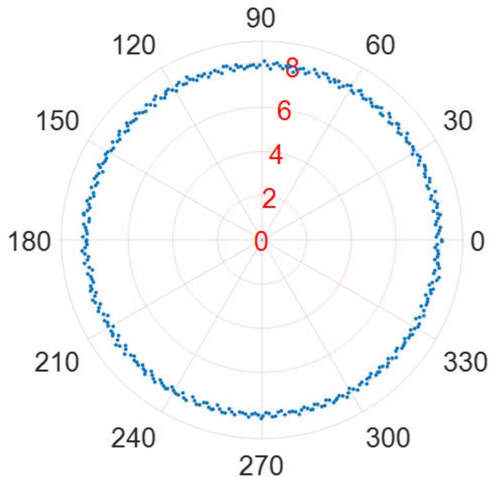
**Figure 6.** The RCS measurement results at the elevation of 0 deg.
