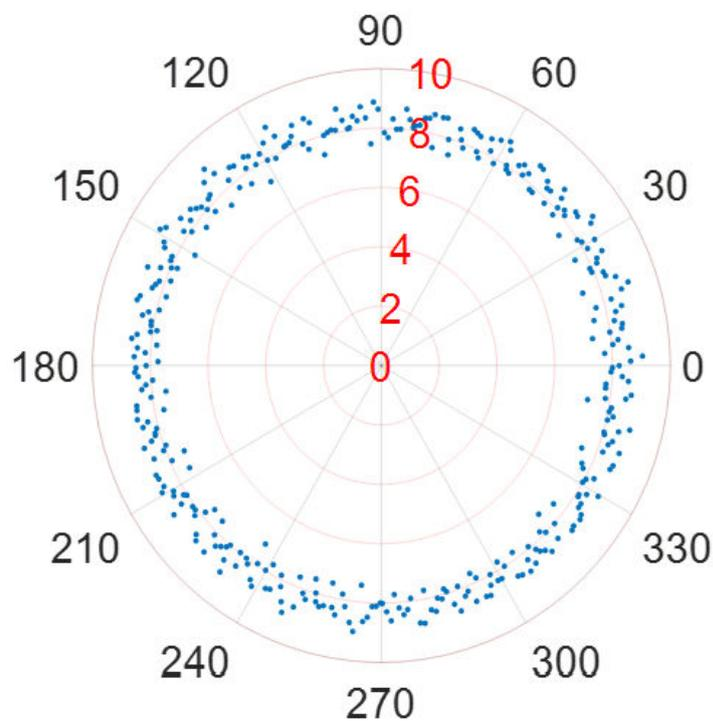
Figure 8. The RCS measurement results at the elevation of 30 deg.
