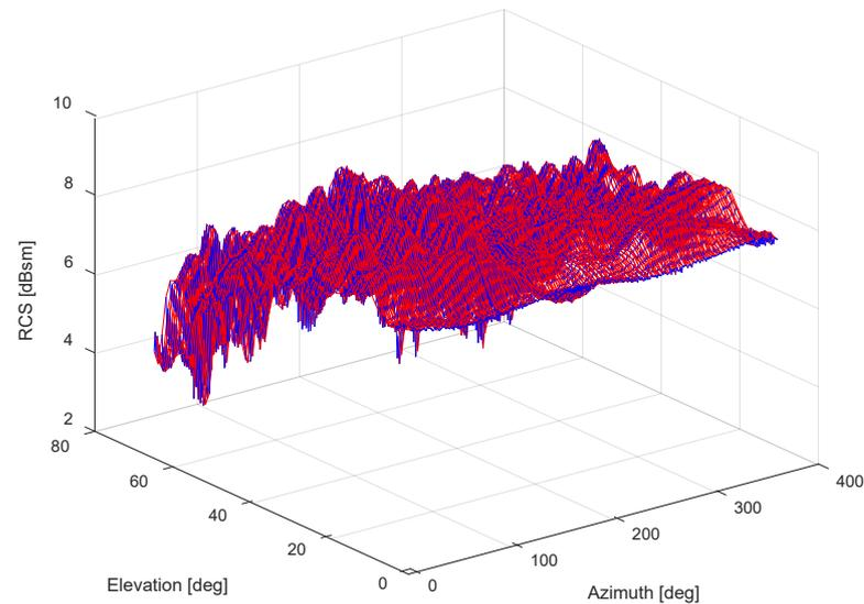
**Figure 5.** The database of laboratory RCS measurements.
