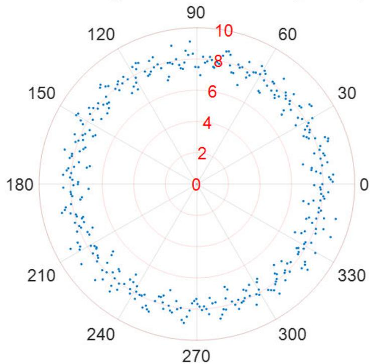
Figure 9. The RCS measurement results at the elevation of 45 deg.
