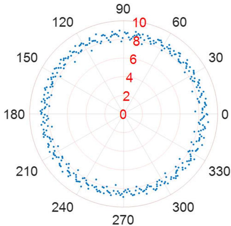
Figure 7. The RCS measurement results at the elevation of 15 deg.
