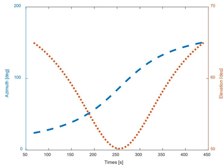
**Figure 11.** The incident orientation of the radar microwave in tracking the spaceborne Luneburg Lens by a ground radar.
