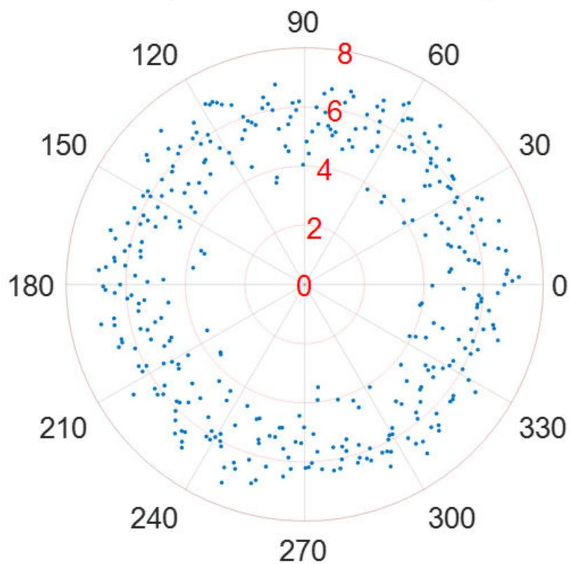
Figure 10. The RCS measurement results at the elevation of 60 deg.
