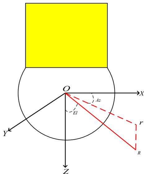
Figure 3. The radar microwave incident angles.
