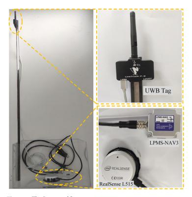
Figure 1. The Layout of Sensors.
