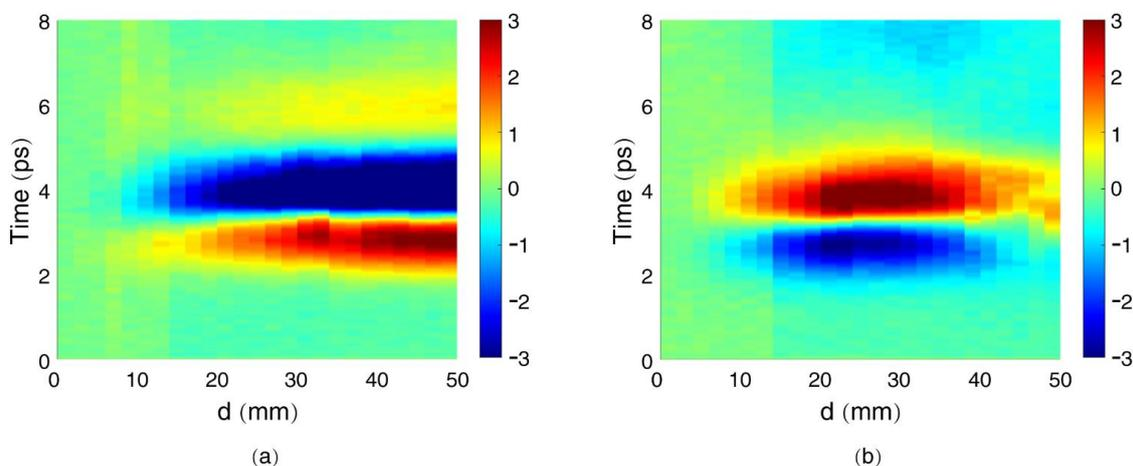
**Figure 5.** Measured THz radiation from a dc-biased filament with a longitudinal external electric field along the filament: (a) horizontally polarized component ( $E_x^{lower}$ ); (b) vertically polarized component ( $E_y^{lower}$ ).
