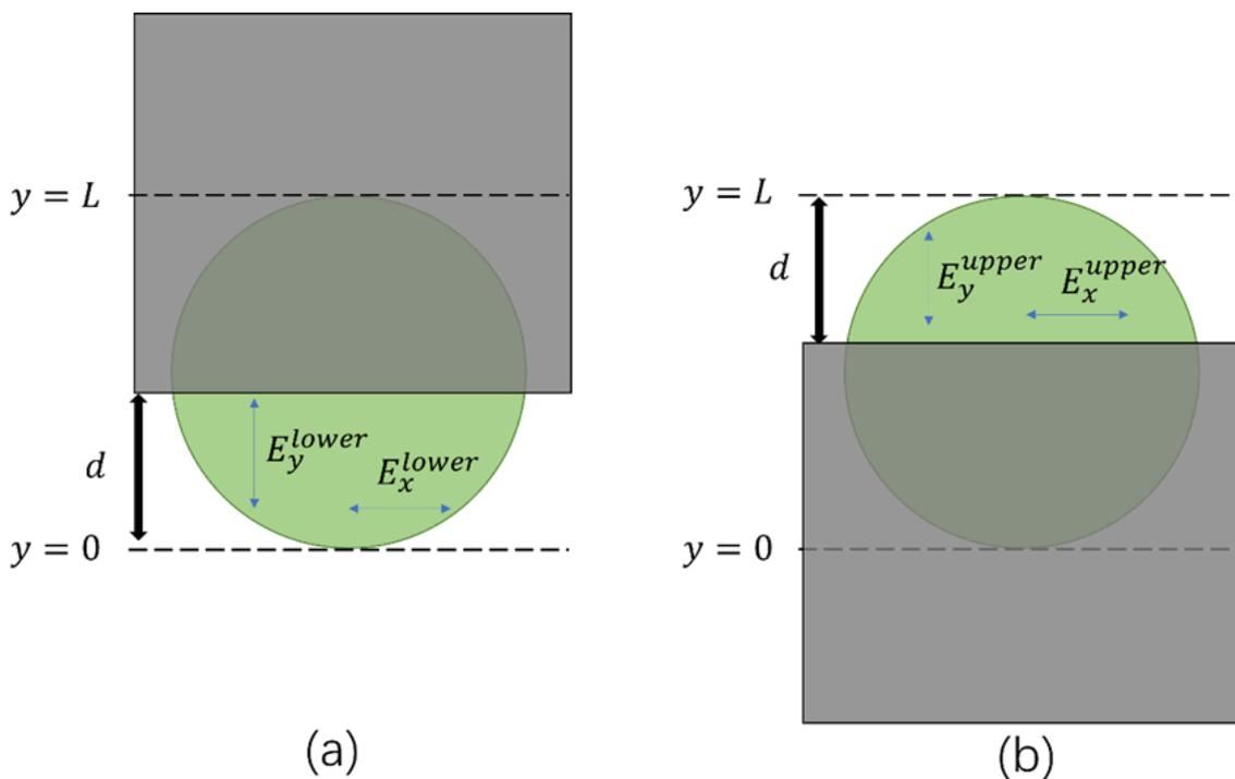
**Figure 3.** Determination of the boundary of the THz beam pattern by moving a metal mask upwards (a), and downwards (b).
