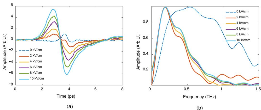
**Figure 8.** (a) Measured waveforms, and (b) corresponding spectra, of the radially polarized THz radiations when the external electric field changes from 0 to 10 kV/cm.
