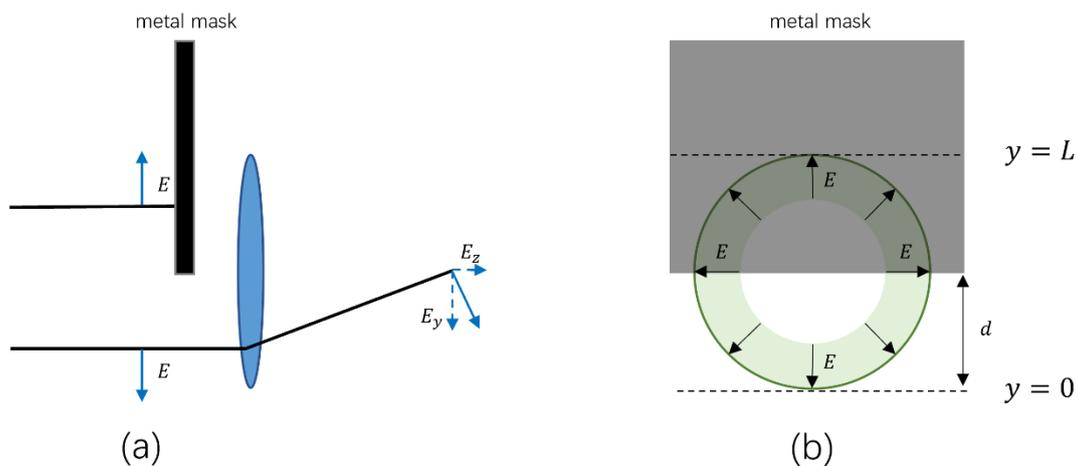
**Figure 2.** Side view (a), and front view (b), of the schematic diagram for beam shielding with a rectangular metal mask.
