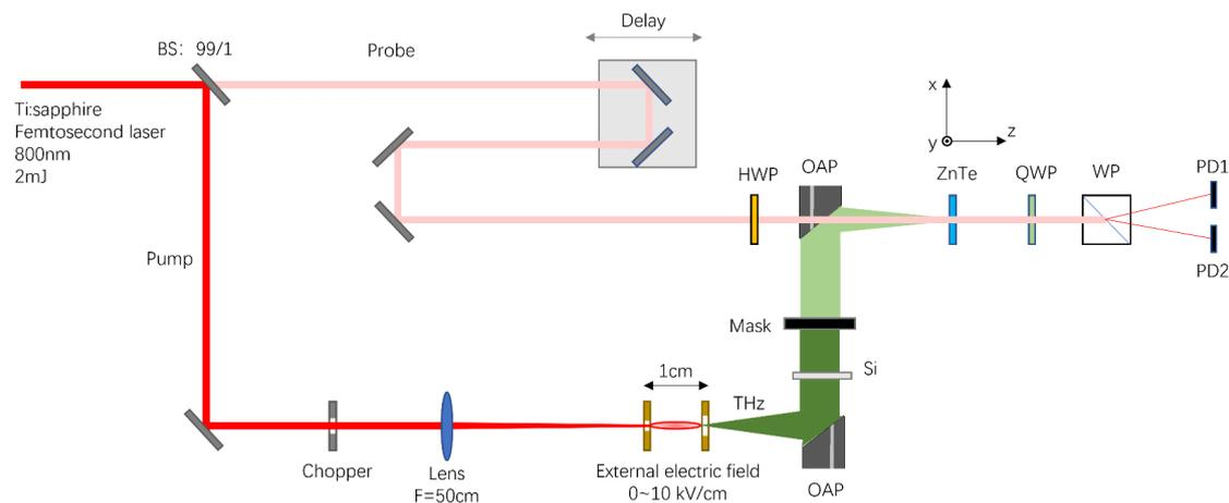
**Figure 4.** Schematic diagram for the experimental setup: HWP, half-wave plate; QWP, quarter-wave plate; WP, Wollaston prism; PD, photodiode detector.
