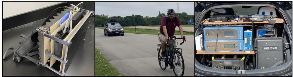
**Figure 4.** Data collection images. (**Left**) custom-made backpack to house biometric devices and recording computer; (**middle**) participant and environmental survey vehicle riding in tandem during data collection; (**right**) environmental sensors organized in trunk of electric survey vehicle.
