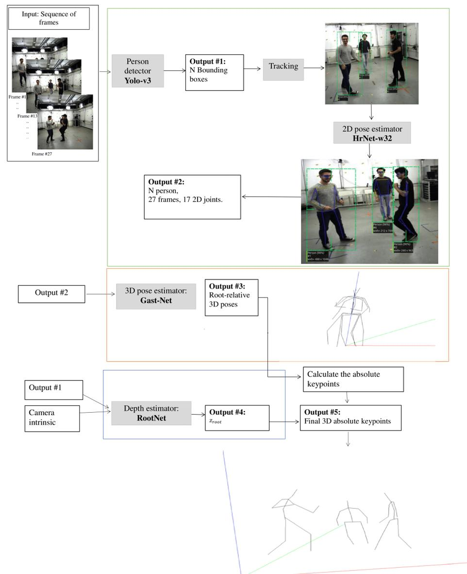
Figure 3. The pipeline of the Root-GAST-Net framework.
