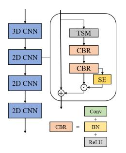
**Figure 3.** The implementation of the residual block in the proposed front-end. As shown in the picture above, in each residual block, the input data will first obtain the short-term time information through TSM. Then, go through the conventional convolution composed of two CBR. Finally, use the SE module to reweight the channel correlation.
