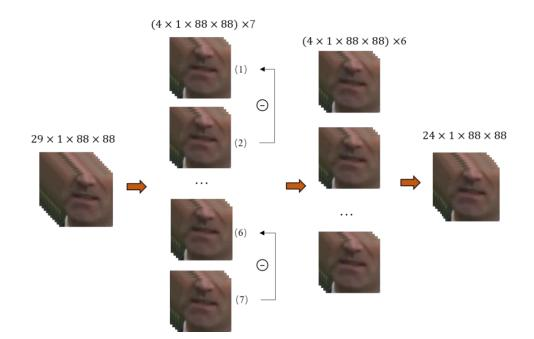
**Figure 5.** Sparse difference sampling. Given a sequence of 29 frames, we divided it into seven segments, each of which is four frames. Then subtract the previous sub-segment from the current sub-segment, for example subtracting sub-segment 1 from sub-segment 2, sub-segment 2 from sub-segment 3, etc. Finally, splice these segments in the temporal dimension to get a 24-frame result.
