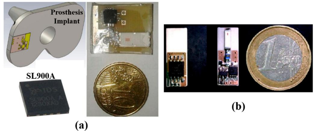
**Figure 10.** (a) Single COTS-based SoC IWMD implant [71] demonstrating fabricated IWMD including antenna and SL900A chip [69]. (b) Demonstration of LORAWAN signal for IWMD built with multiple COTS [72].
