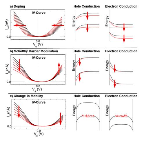
**Figure 6.** Theoretical I-V curves of a chemFET depending on (**a**) the doping (**b**) Scottky barrier modulation (**c**) change in mobility. Reprinted with permission from [15]. Copyright (2018) from American Chemical Society.
