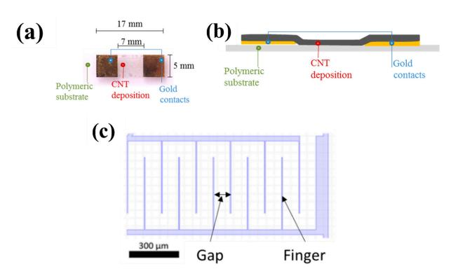
**Figure 3.** (a) Top view and (b) cross section of an example of two terminal resistive CNT sensors on ETFE (Ethylene Tetra Fluoro Ethylene). Reproduced from [92]. (c) Schematic of interdigitated electrodes.
