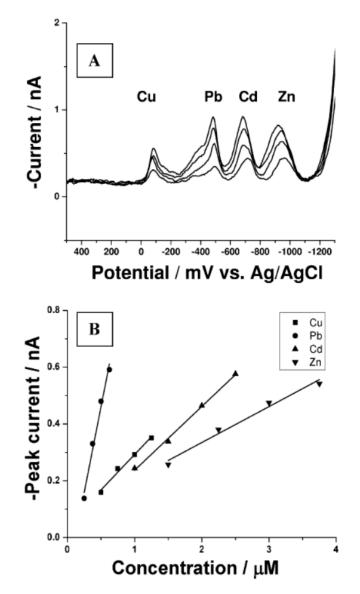
**Figure 7.** (A) Simultaneous detection of Cu(II), Pb(II), Cd(II) and Zn(II), ion concentrations 0.5, 0.25, 1.0, 1.5  $\mu$ M for Cu(II), Pb(II), Cd(II), Zn(II), respectively; and 1.5, 2, 2.5 times of above concentrations for these metals ions. (B) Calibration Curve for Cu(II), Pb(II), Cd(II), Zn(II). Accumulation time: 120 s, deposit potential: -1.5 V. Reproduced from [129].
