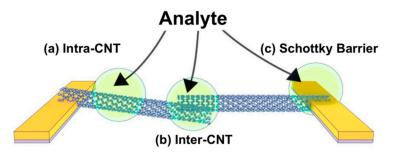
**Figure 5.** Schematic of possible sensitivity sites which affect the conductivity: (**a**) at the sidewall or along the length of the CNT itself, (**b**) interface between CNT-CNT (inter-CNT) and (**c**) at the interface between the metal electrodes and the CNT (Schottky barrier). Reprinted with permission from [15]. Copyright (2018) from American Chemical Society.
