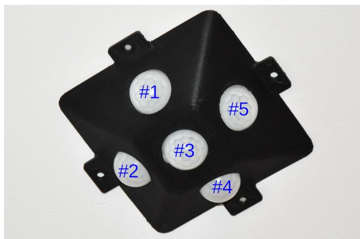
**Figure 2.** Sensor module with passive infrared (PIR) sensors.
