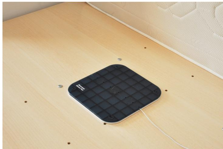
**Figure 1.** Piezoelectric-based sensor placed under the mattress to detect movements in bed.
