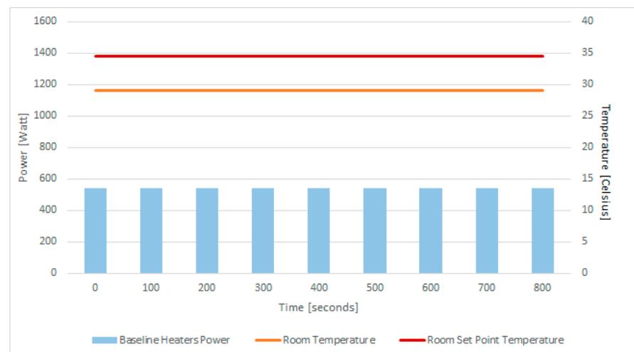
**Figure 8.** Initial conditions: the 4 QRad server heaters' total power demand and initial temperatures.
