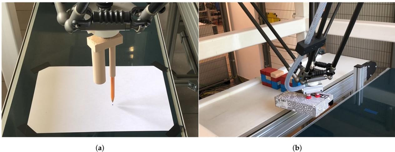
Figure 8. General view of IRB360 robot with: (a) pen; (b) suction gripper carrying a detail.
