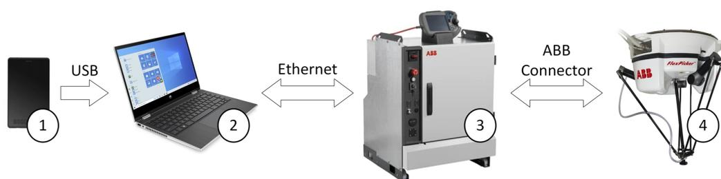
**Figure 1.** General station view: 1—Huion graphics tablet, 2—PC, 3—IRC5 controller, 4—IRB 360 industrial robot.
