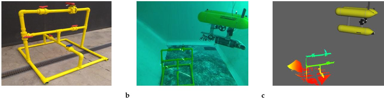
**Figure 11.** Image of the Girona 500 AUV inspecting the structure. The mapped structure before deployment (a), underwater view of the water tank (b) and online 3D visualizer with a scan of the structure (c).
