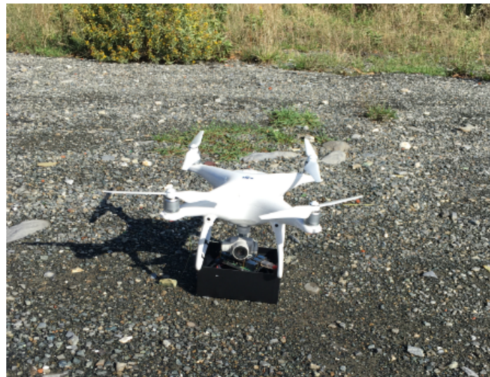
Figure 7. UAV equipped with an IoT LoRaWAN gateway.
