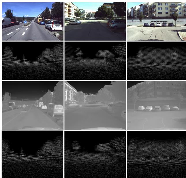
**Figure 7.** Example of a depth map created by reprojection of point cloud data into the RGB and thermal camera frames. First row—RGB image; second row—corresponding depth map; third row—thermal image of the same scene; fourth row—depth map projected into the thermal camera frame.
