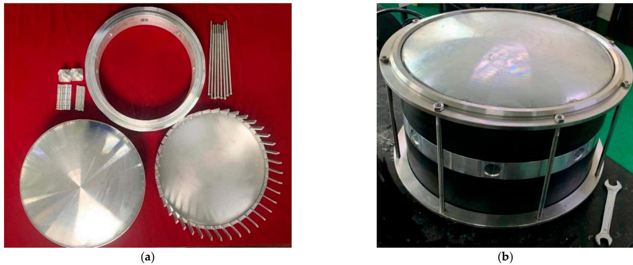
**Figure 13.** (a) Assembling components of transducer. (b) Fully assembled transducer.
