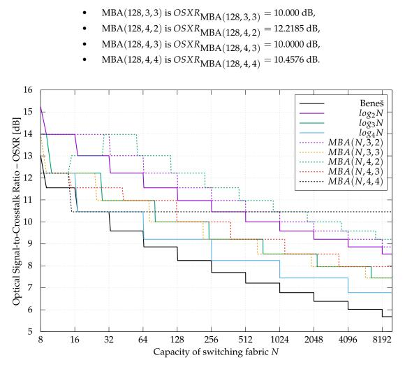
Figure 10. Optical signal-to-crosstalk Ratio (OSXR) for different switching fabrics.
