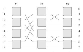
Figure 1. The banyan switching fabric of 8 inputs and 8 outputs (also called the log<sub>2</sub> 8 switching fabric).
