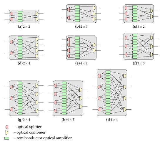
Figure 4. Optical switching elements (OSE) of different sizes.
