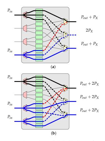
**Figure 9.** The optical crosstalk (dashed) in the OSE of size  $4 \times 3$ . (a) with the considered connection (solid black) and one intersecting connection (solid blue); (b) with the considered connection (solid black) and two intersecting connections (solid blue).
