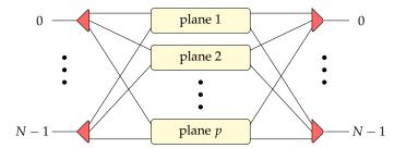
Figure 2. The idea of a multiplane switching fabric.
