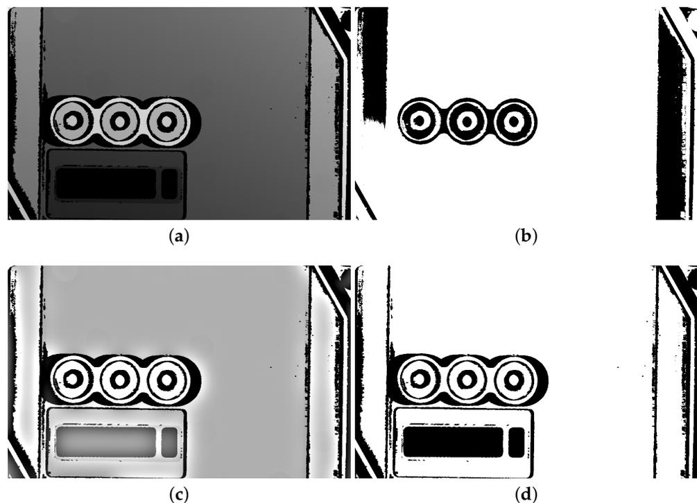
**Figure 3.** Retinex filter. (a) The scanned depth map; (b) binarization of the scanned depth map by the IsoData threshold; (c) the output from the Retinex filter applied to the scanned depth map; (d) binarization of the Retinex filter output by the IsoData threshold.
