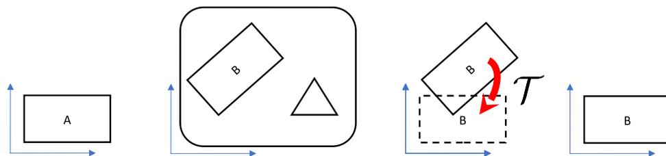
**Figure 1.** The objects recognition and alignment tasks. From left to right: template, scan, the recognized object with transform, the aligned object (top view of 3D scenes).
