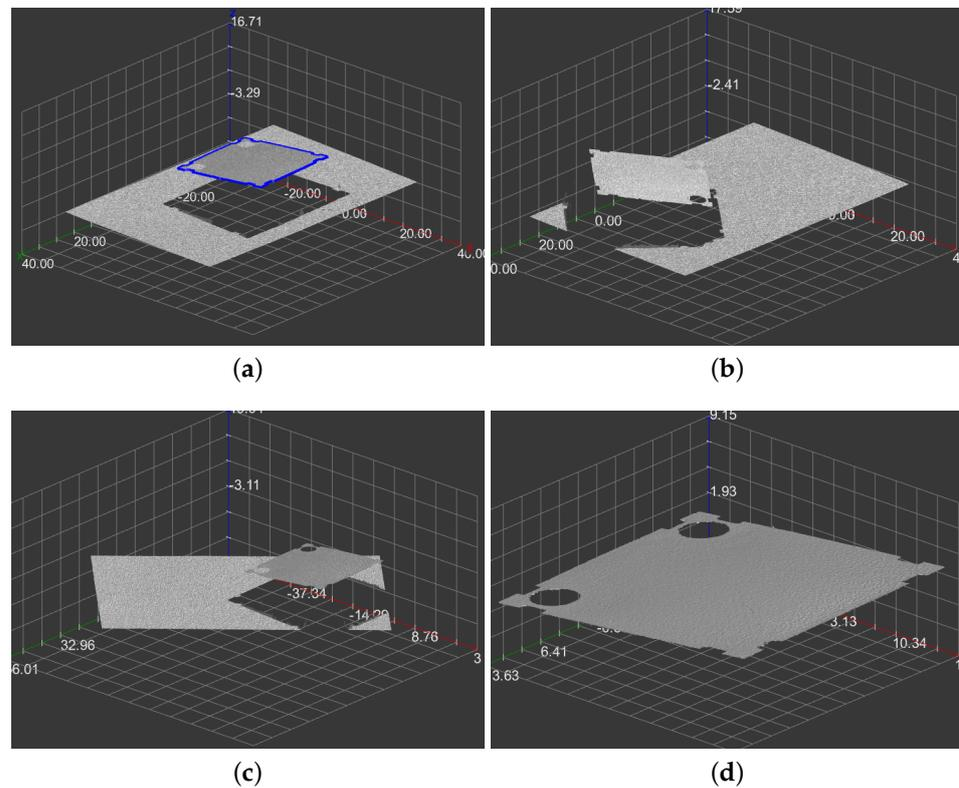
**Figure 8.** Results for a single input. (a) Contour selected for the template; (b) the input depth map; (c) the aligned depth map; (d) the recognized and aligned object.
