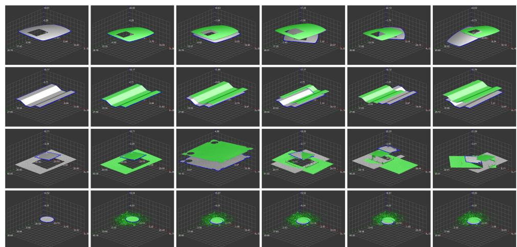
**Figure 9.** Here, we present results for several objects and their scans. Each line offers five scans of the same item, from which the first one we select as the template (the first column). The gray color represents measured values while the green one the aligned depth map (we align the whole depth map for better comparison; the recognized object could also be separated, of course).
