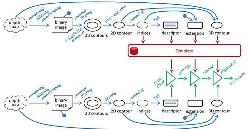
**Figure 2.** Our processing pipeline for object recognition and alignment.
