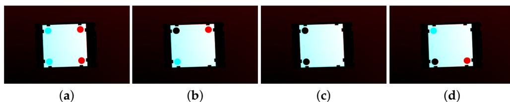
**Figure 5.** An example of an object with symmetric shape and asymmetric aspects. (a–d) Aligning by the outer shape, there are four possible alignments, but only one (c) is correct. (The template object is cyan, and the aligned one is red. Thus pure cyan represents a missing area and pure red an extra area.)
