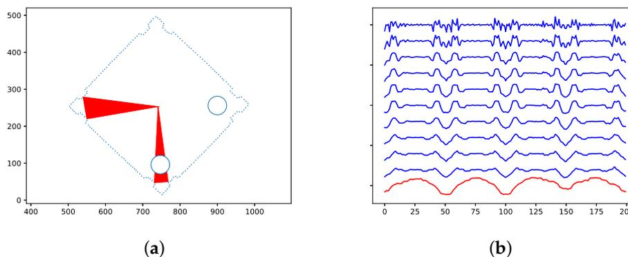
**Figure 6.** Extension of the TAR descriptor. (a) the sampled contour and holes with examples of triangle areas describing the inner object area. (b) the TAR descriptor with our extension (the bottom line). It is quite visible that the standard TAR values contain four same segments, whereas the extension two plus two. Thus alignment is uniquely determined.
