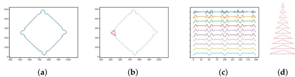
**Figure 4.** Shape descriptor based on the Triangle Area Representation (TAR). (a) Contour; (b) sampled contour (200 points) with an example of the considered triangle; (c) TAR descriptor (each line represents 200 normalized triangle areas; each area corresponds to point and its close neighbors) (d) illustrative triangles (indicating how far the neighbors are from the point).
