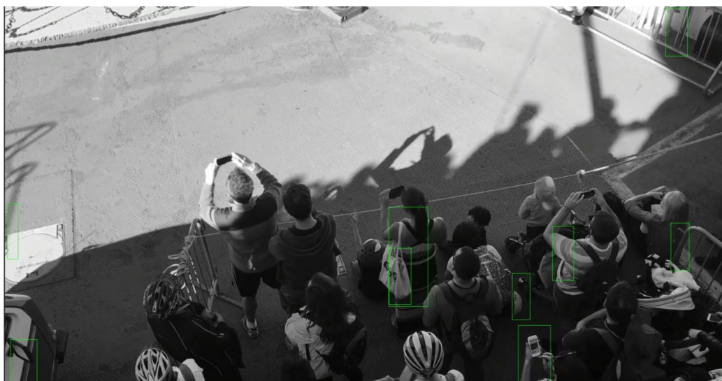
Figure 3. Screenshot of video stream being analyzed by the Python script and its division into labeled cells.
