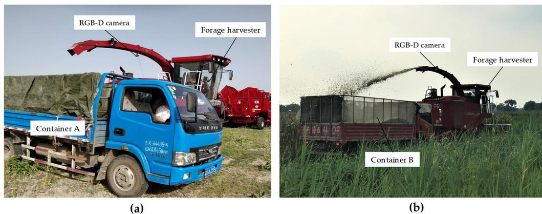
**Figure 5.** The identification and positioning experiments with different trucks. (a) Container A is heightened by welding steel and covered by a tarpaulin. (b) Container B is modified from the high-strength mesh.
