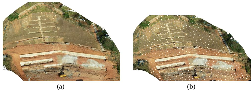
**Figure 16.** Inspection site: (a) 3D model; (b) waypoints.
