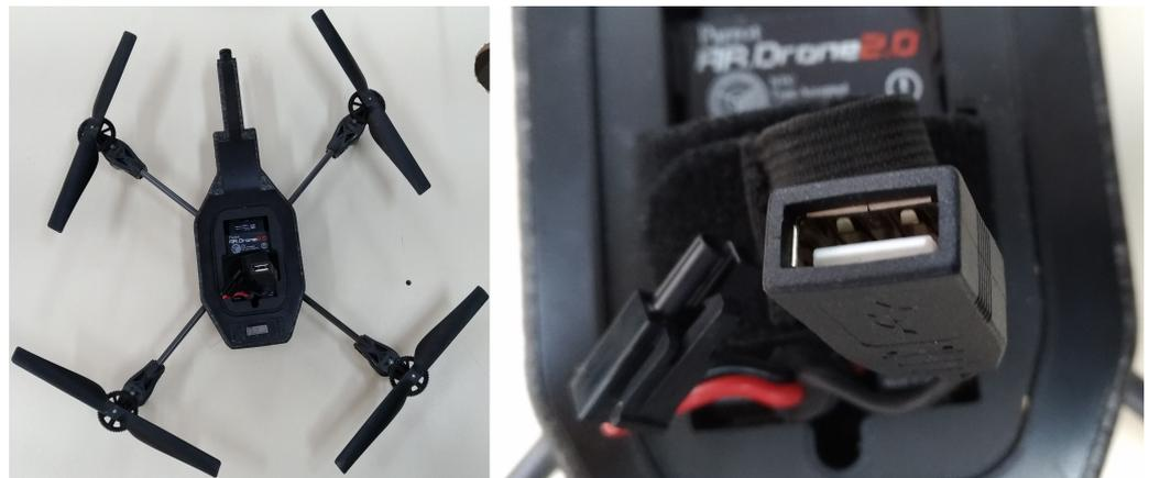
**Figure 7.** The Parrot AR.Drone 2.0 without its hull, highlighting its USB port.
