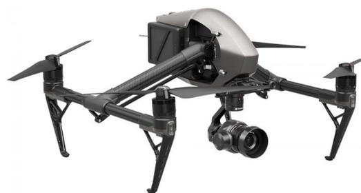
**Figure 1.** DJI Inspire 2, a mini UAV weighing around 3.3 kg and capable of a flight time up to 27 min [17].
