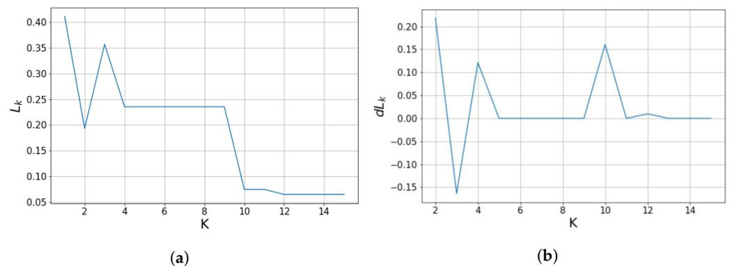
**Figure 3.** (a) Average cosine-distance value of a point cloud calculated by Equation (4) according to  $K$ , the number of planes. (b) Difference of average cosine-distance calculated by Equation (7). If  $K$  is sufficient to cluster point cloud into planes, we can see that the difference of average cosine-distance converges close to zero and no longer changes. By using difference of average cosine-distance, we can obtain the appropriate parameter  $K$ .
