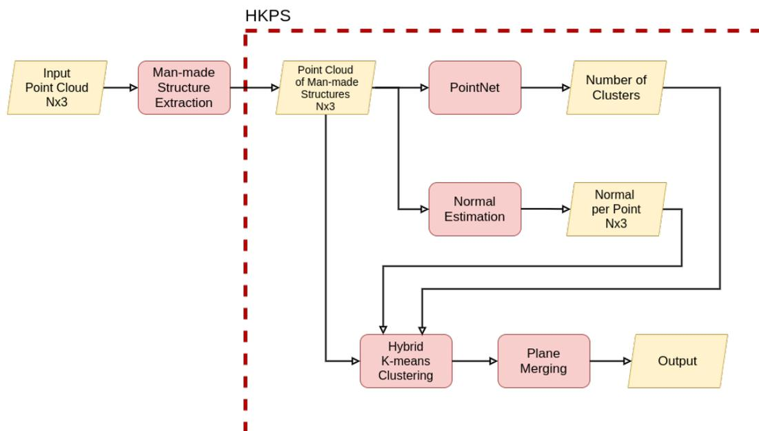
**Figure 2.** An overview of the proposed framework. PointNet [6] takes the input point cloud of man-made structure and outputs the number of clusters. We estimate the normal of each point, and then perform hybrid K-means clustering for plane segmentation (Sections 3.1 and 3.2). At the end of the network architecture, the plane merging process optimizes the number of planes (Section 3.3).
