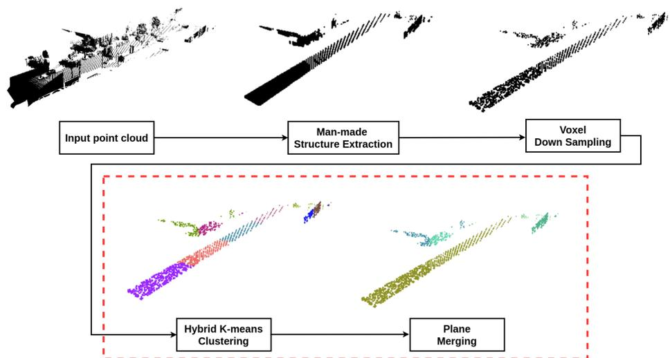
**Figure 1.** The plane segmentation procedure using the proposed system. We extract man-made structures from the unorganized input point cloud and voxelize the points using voxel down sampling as pre-processing. Then, the proposed hybrid K-means clustering method segments the point cloud into planes. Finally, the merging process combines the small planes that need to be merged.
