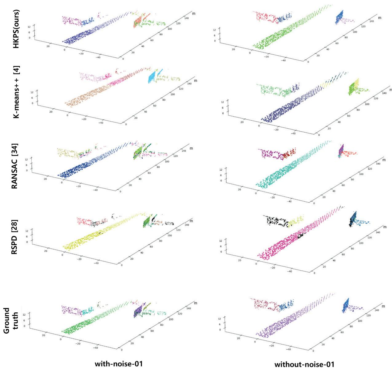
**Figure 5.** Performance comparison results using scene 01 from *with-noise* Virtual KITTI Dataset and *without-noise* Virtual KITTI Dataset. Different planes are displayed with different colors. The outliers of RANSAC and RSPD are colored in black.
