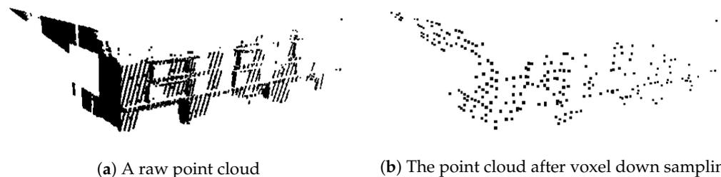
**Figure 4.** The same point cloud (a) before and (b) after voxel down sampling. The density of the point cloud becomes uniform and noise is removed.
