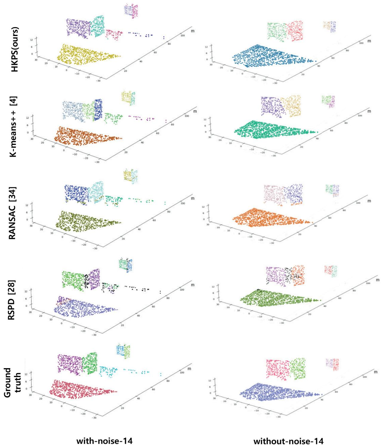
**Figure 6.** Performance comparison results using scene 14 from *with-noise* Virtual KITTI Dataset and *without-noise* Virtual KITTI Dataset. Different planes are displayed with different colors. The outliers of RANSAC and RSPD are colored in black.
