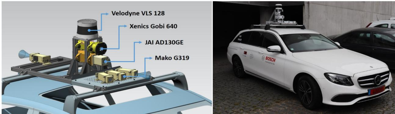
**Figure 1.** A 3D render of the test car sensor setup (left), Final setup installed on the test car (right).
