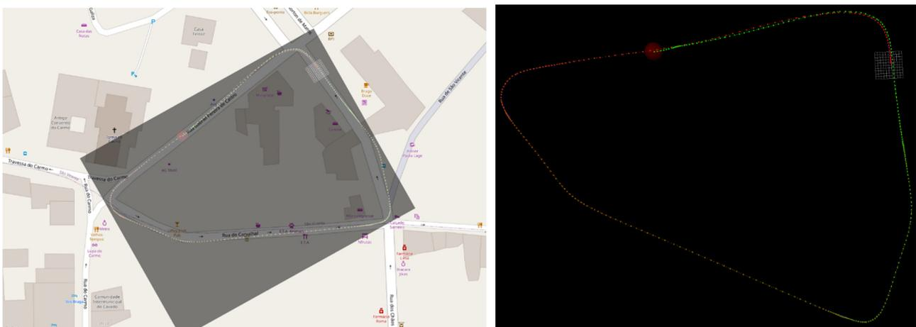
**Figure 13.** Example of a driving sequence: (left) Manual overlap of map view with computed vehicle positions in the map; and (right) Driving sequence featuring the loop, displaying only the estimated vehicle positions.
