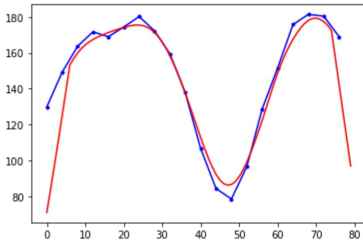
**Figure 7.** An example of data smoothing using discrete linear convolution.
