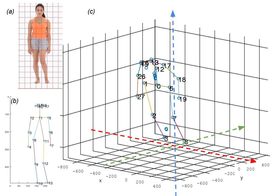
**Figure 14.** An example of 2D and 3D key joint estimation. (a) Input image. (b) The 2D estimation result from the input image. (c) The 3D estimation from the 2D key joints.
