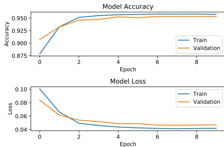
**Figure 16.** The training graphs for the Siamese-LSTM network with CASIA-A. The graph shows the training was successful with around 95% accuracy and 0.04 loss after 10 epochs.
