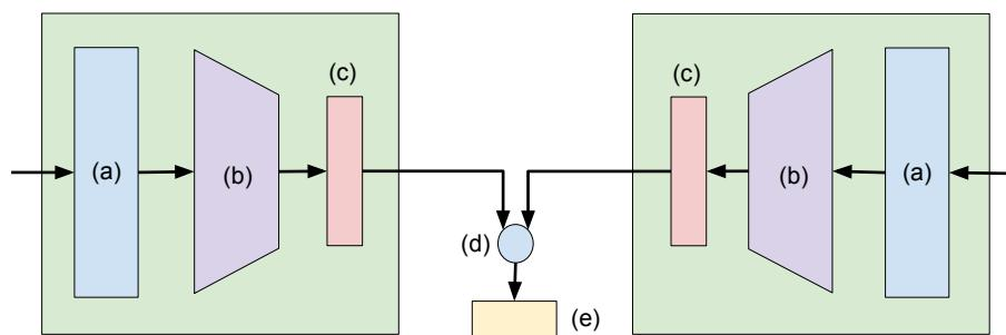
**Figure 9.** Siamese Neural Network with two identical subnetworks. (a) Input (b) Convolutional Neural Network layers (c) Fully connected—sigmoid layer (d) Absolute difference (e) Fully connected—sigmoid layer.
