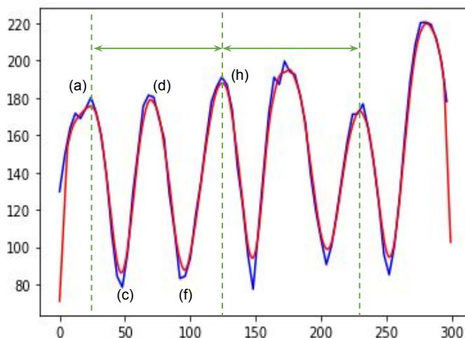
**Figure 6.** Gait cycle extraction in a sample of  $d_t(a)$ . One gait cycle (green solid line arrows) is from the changes in the distance of two ankles. To remove a subtle change in these ankle distances, data smoothing is applied. The line in blue is raw data. The line in red is after smoothing. The  $x$ -axis is for the image frame numbers. The  $y$ -axis is for the 3D distances between the two joints.
