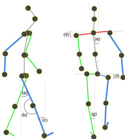
**Figure 8.** Angle features. (a) Hip extension angle, (b) Knee flexion angle, (c) Leg inclination angle, (d) Lateral shoulder drop angle, (e) Trunk side bending angle, (f) Lateral pelvic drop angle, (g) Rearfoot eversion angle.
