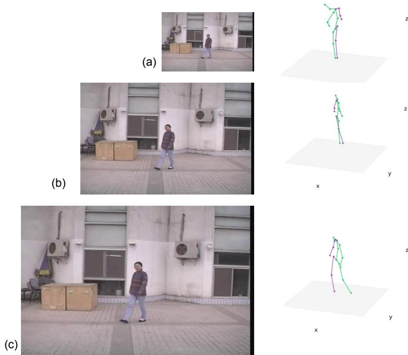
**Figure 21.** The test with scale-up images that shows a better 3D pose estimation. (a) The original image size  $352 \times 240$ . The 3D estimation result shows some deformation (b) The scaled image to  $704 \times 480$ . No more severe deformation is found. Yet, it is not enough to extract gait features (c) The scaled image to  $1126 \times 768$ . The human subject size is roughly  $100 \times 250$  which is big enough as an input to 2D and 3D pose estimator.
