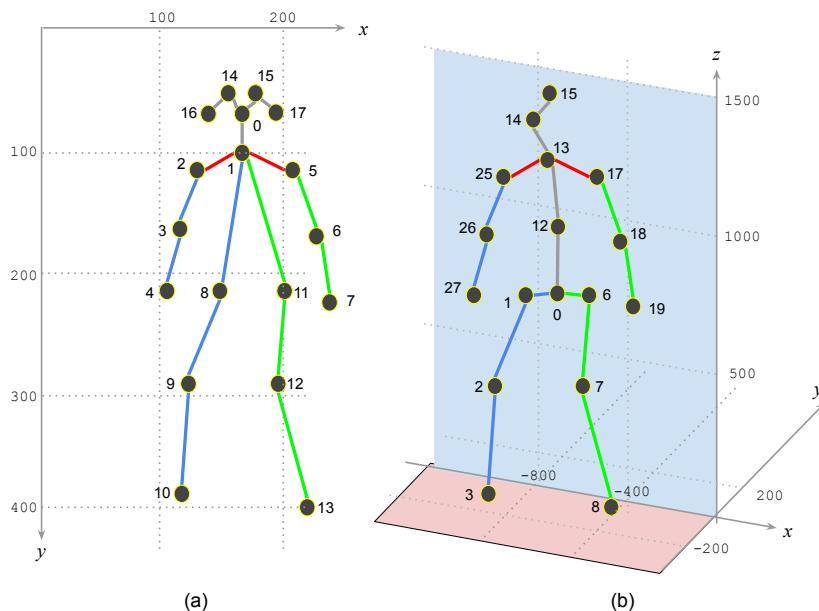
**Figure 4.** The coordinate system difference between (a) OpenPose. The joint positions are labeled in 2D locations. (b) SYEB. The joint positions are in 3D. The depth information is inferred by the embedded 3D joint position estimator.
