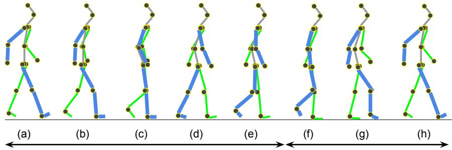
**Figure 5.** Human gait cycle. (a) Initial contact, (b) Loading response, (c) Mid-stance, (d) Terminal stance, (e) Pre-swing, (f) Initial swing, (g) Mid-swing, (h) Terminal swing. The stance phase is defined from (a) to (e). The swing phase is from (f) to (h). The initial contact and the terminal swing is the same event with a different name.
