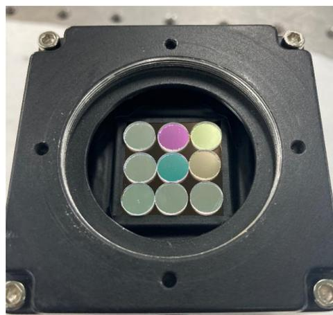
**Figure 12.** Multispectral coding aperture lensless imaging prototype.
