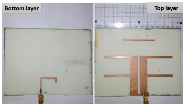
**Figure 1.** (a) The antenna element structure; (b) the antenna prototype.
