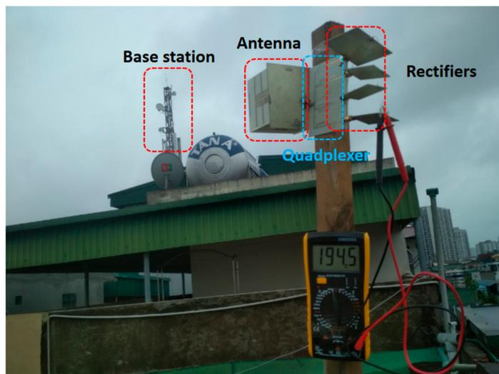
Figure 14. Experimentation of the proposed multiband rectenna.
