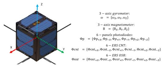
Figure 1. Spacecraft body frame of the UVSQ-SAT satellite.
