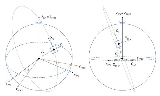
**Figure 5.** Earth-centered inertial (ECI), Earth-centered Earth-fixed (ECEF), and orbit (O) reference frames.
