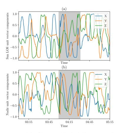
**Figure 9.** First lights of the Sun LOS (**a**) and nadir (**b**) components in the satellite body frame based on MEKF on 2 March 2021 (representative period in the case of measurements at 30 s intervals almost continuously with eclipse phase in gray).
