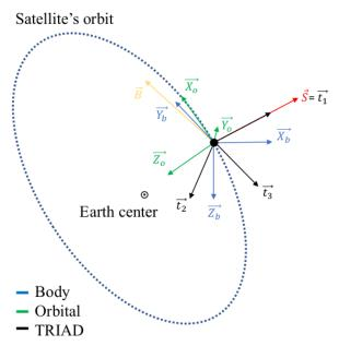
Figure 7. Reference frames for TRIAD method.
