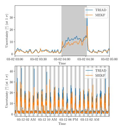
**Figure 14.** Uncertainties estimated from the Monte Carlo method for TRIAD and MEKF methods for continuous sampling on 2 March 2021 (**top**) and from 11–13 March 2021 (**bottom**) with eclipse phases in gray.
