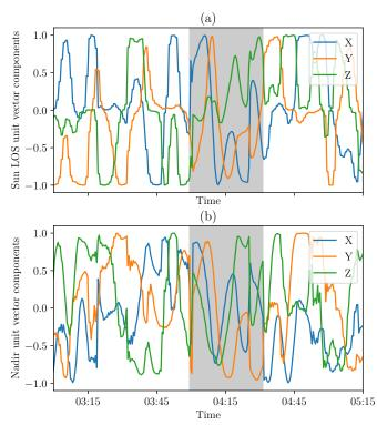
**Figure 8.** First lights of the Sun LOS (a) and nadir (b) components in the satellite body frame based on TRIAD method on 2 March 2021 (representative period in the case of measurements at 30 s intervals almost continuously, with eclipse phase in gray).
