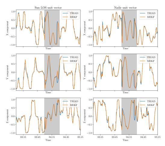
**Figure 10.** First lights of the Sun LOS and nadir coordinates in the satellite body frame based on MEKF and TRIAD on 2 March 2021 (representative period in the case of measurements at 30 s intervals almost continuously with eclipse phase in gray).
