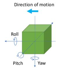
Figure 6. Euler angles defined for the satellite.
