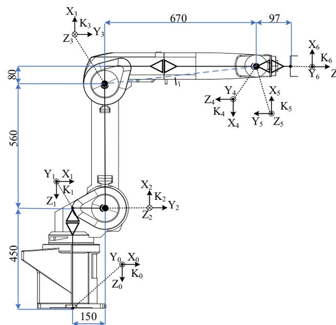
**Figure 8.** Mitsubishi RV-12sl industrial robot's overall dimensions.
