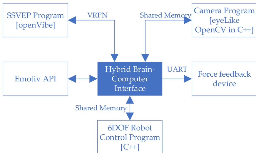
Figure 3. Structure of hybrid brain-computer interface software.
