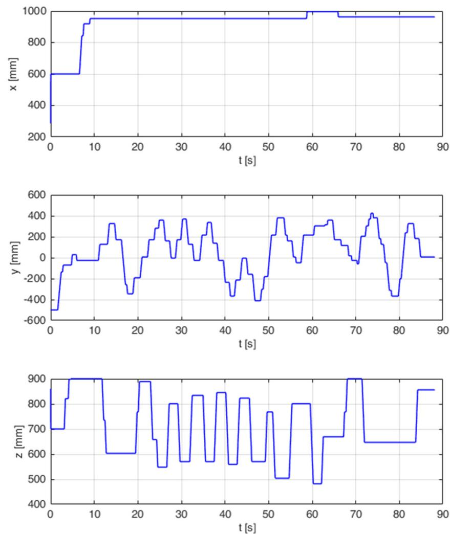
**Figure 17.** End points of real robot tip positioning endpoints when trying to sort.
