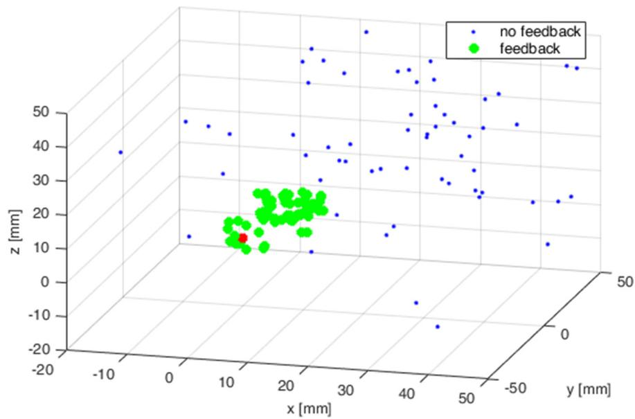
**Figure 14.** End points of robot tip positioning with enabled and disabled feedback.
