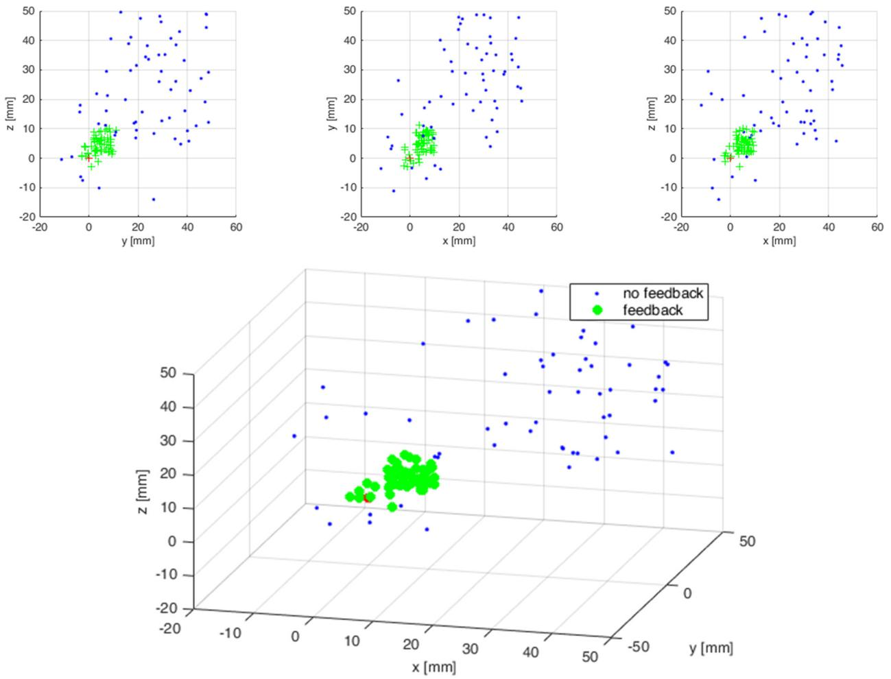
Figure 13. End points of virtual robot tip positioning with enabled and disabled feedback.
