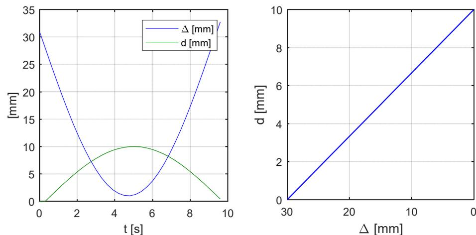
Figure 7. Plot of block extension and distance of robot tip from the box versus time (left) and plot of block extension versus distance of robot tip (right).
