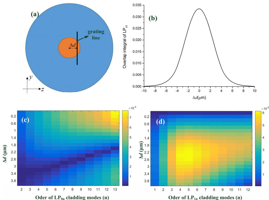
**Figure 5.** (a) Schematic of a cross-section of LBL-FBG. (b) Overlap integral of LP<sub>01</sub> versus offset distance ( $\Delta d$ ). (c) Overlap integral of LP<sub>0n</sub> cladding modes versus offset distance ( $\Delta d$ ). (d) Overlap integral of LP<sub>1n</sub> cladding modes versus offset distance ( $\Delta d$ ).
