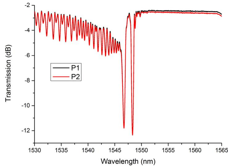
**Figure 4.** Transmission spectra of LBL-FBG2 under two different polarization states.
