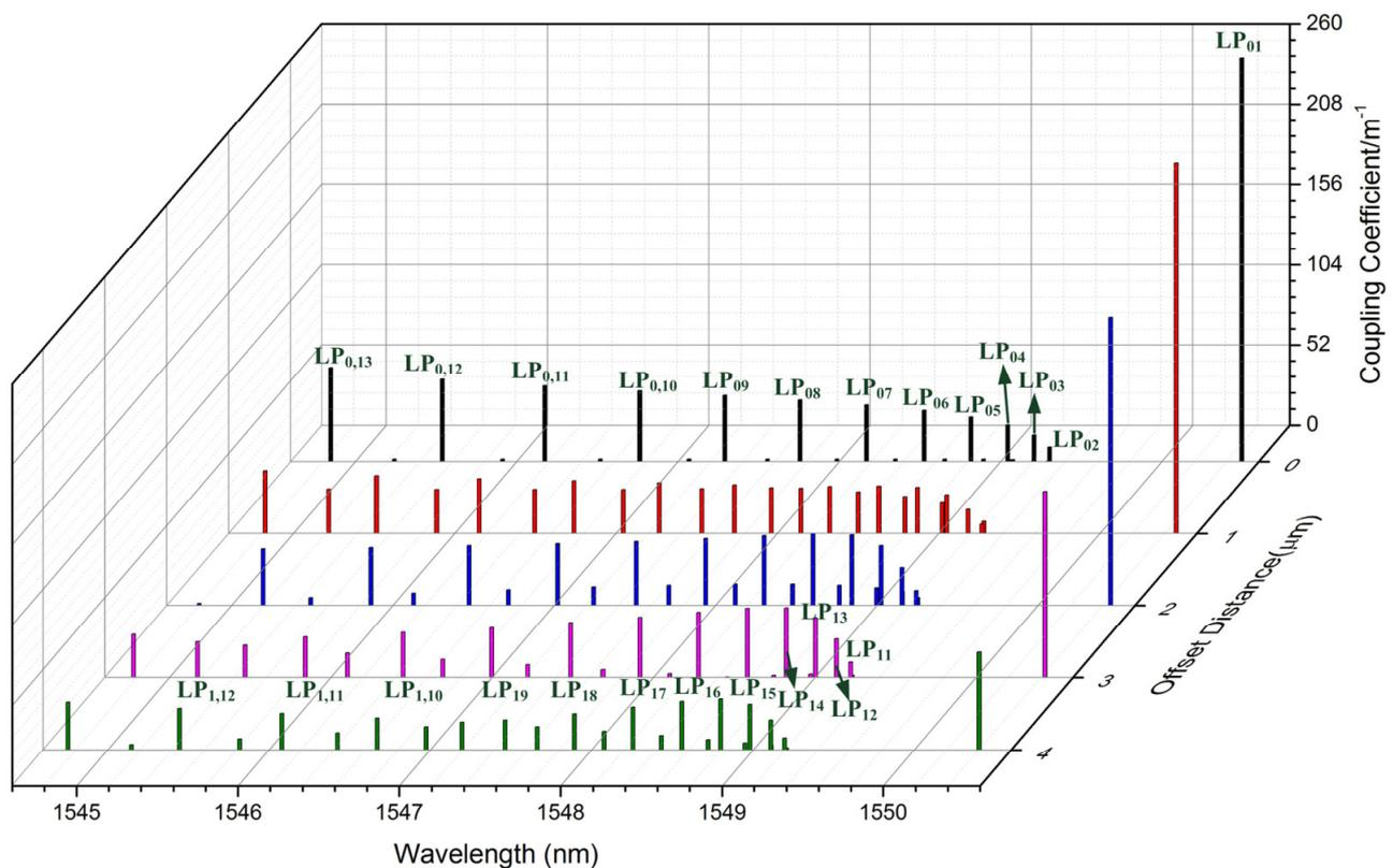
Figure 6. Coupling coefficients of LBL-FBG with different offset distance ( $\Delta d$ ).
