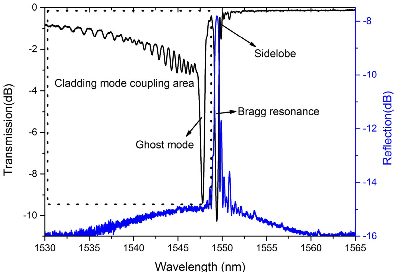
Figure 2. Typical spectrum of LBL-FBG (black-dotted-bordered rectangle represents the cladding mode coupling area).
