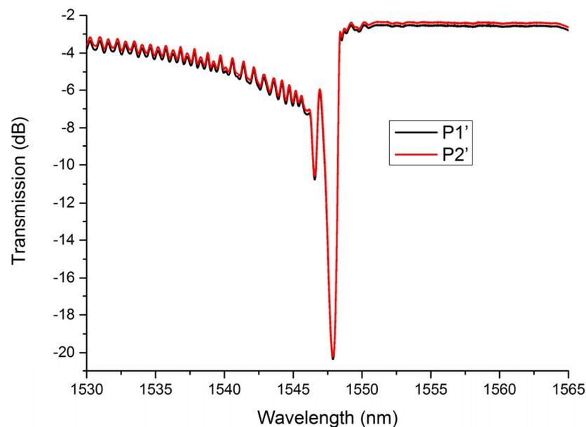
**Figure 9.** Transmission spectra of apodized LBL-FBG under different polarization states.
