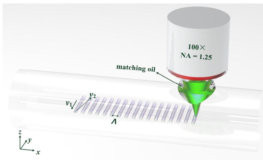
**Figure 1.** Inscription schematic of LBL-FBGs with oil-immersion lens.
