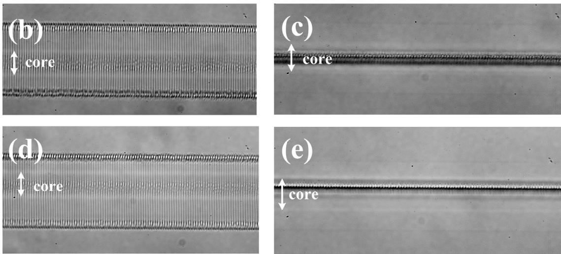
**Figure 3.** (a) Transmission spectrum of LBL-FBG1 and LBL-FBG2. Microscopy image (100 $\times$ ) of LBL-FBG1: (b) top view and (c) side view. Microscopy image (100 $\times$ ) of LBL-FBG2: (d) top view and (e) side view.
