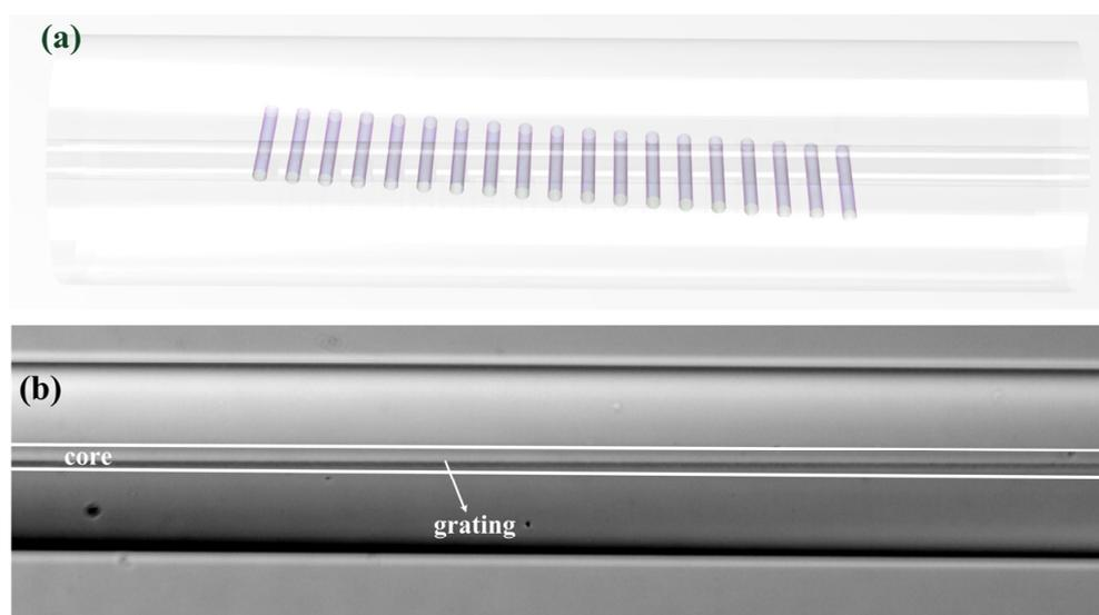
**Figure 7.** (a) Schematic of apodized LBL-FBG. (b) Microscopy (10 $\times$ ) of apodized LBL-FBG.
