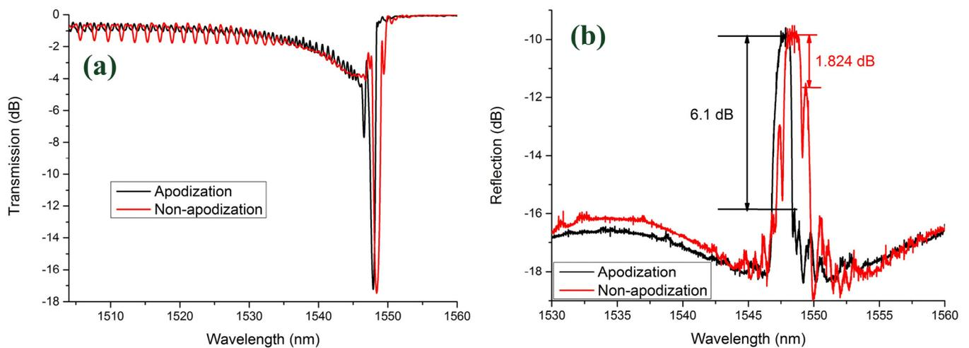
**Figure 8.** Comparison between apodized LBL-FBG and non-apodized LBL-FBG: (a) transmission spectrum and (b) reflection spectrum.
