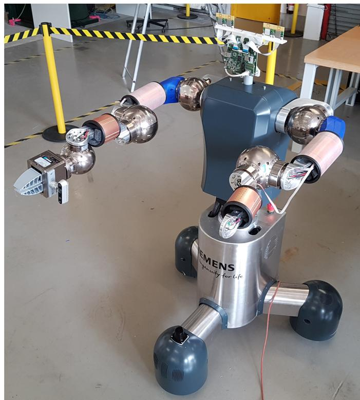
**Figure 2.** Smart capacitive sensor skin mounted on a robot. Two skin sensors are mounted on the lower arm, two on the upper arm respectively.
