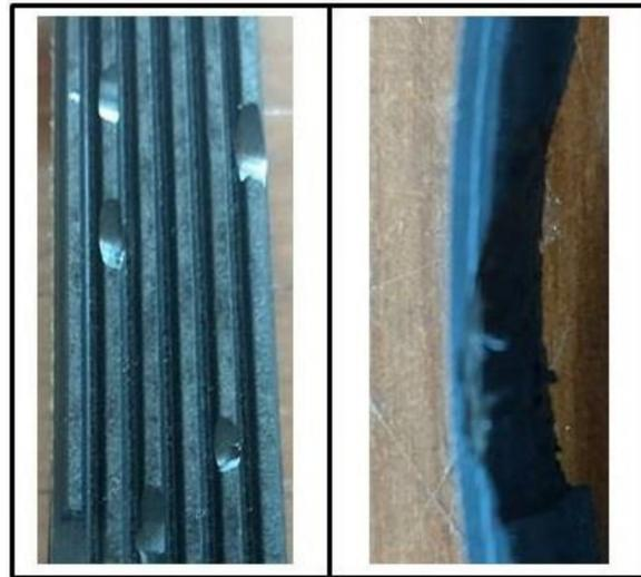
**Figure 9.** BPD fault (left) and BCL fault (right).
