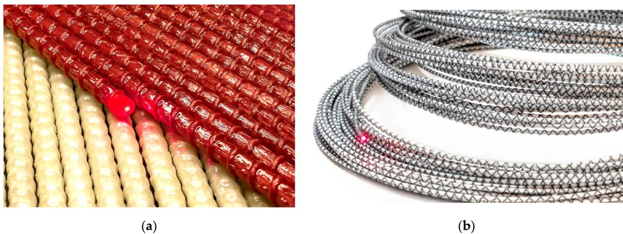
**Figure 8.** Sensors used in the monitoring system. (a) Sensor A—EpsilonRebar, (b) Sensor B—EpsilonSensor [8].
