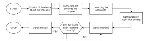
Figure 4. Block diagram describing the operation of the application.
