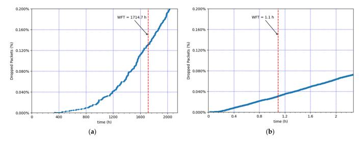
**Figure 7.** Evolution of cumulative packet drops at the EDs due to duty cycle restrictions over time. (**a**) Lowest load: 30 CEDs, using an EDL of 0.9 packets/h. (**b**) Highest load: 100 CEDs, using an EDL of 18 packets/h.
