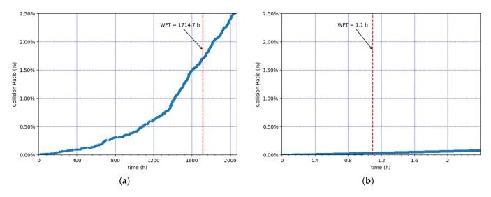
**Figure 6.** Evolution of cumulative collisions at the gateway over time. (a) Lowest load: 30 CEDs, using an EDL of 0.9 packets/h. (b) Highest load: 100 CEDs, using an EDL of 18 packets/h.
