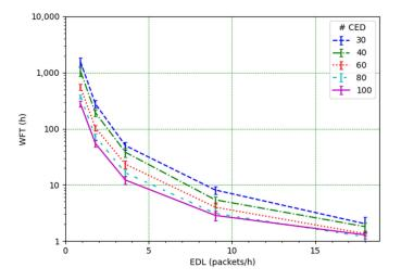
Figure 9. Mean and standard deviation of WFT as a function of EDL, for several numbers of CEDs.
