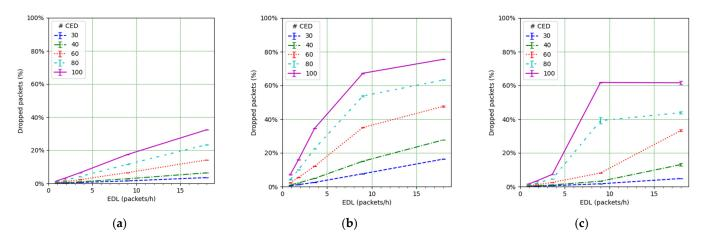
Figure 17. Packet losses due to duty cycle at the gateway vs. EDL for (a) SFM1, (b) SFM2, and (c) SFM3.
