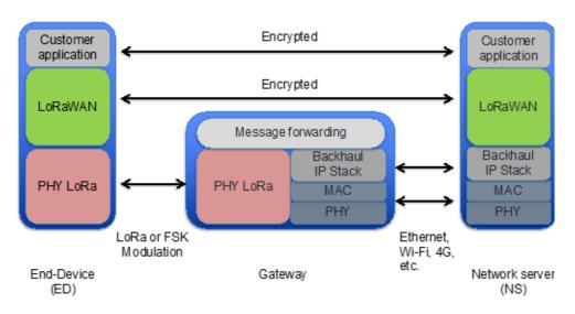
Figure 1. LoRaWAN protocol stack for each network element.
