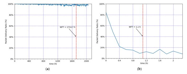
**Figure 8.** Instantaneous PDR after WFT. (**a**) Lowest load: 30 CEDs, using an EDL of 0.9 packets/h. (**b**) Highest load: 100 CEDs, using an EDL of 18 packets/h.
