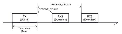
**Figure 2.** Uplink transmission followed by the two receive windows, RX1 and RX2, defined in LoRaWAN class A.
