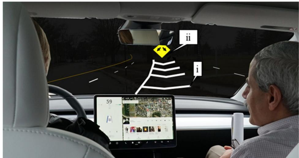
**Figure 3.** Level 2 autonomous vehicle tracking on an interstate. Available online: <https://youtu.be/6QCF8tVqM3I> (accessed on 1 October 2020).
