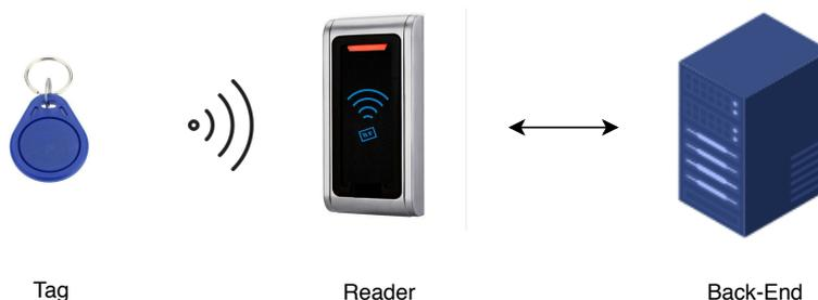
Figure 1. RFID components.
