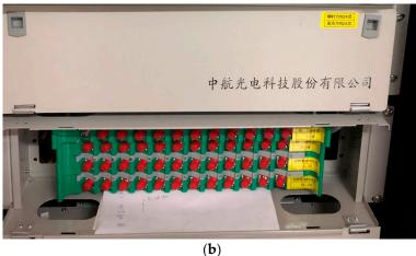
**Figure 4.** (a) The hardware and software of the  $\Phi$ -OTDR system; (b) The sensing fiber-optic cable distribution frame.
