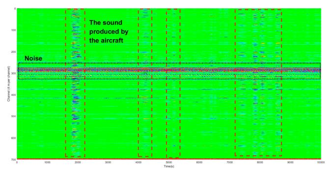
**Figure 5.** Original signal of an airplane.
