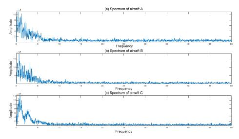
$\label{eq:Figure 7.} \textbf{Figure 7.} \ \textbf{The spectrums of seismic vibration signals from the three aircraft.}$
