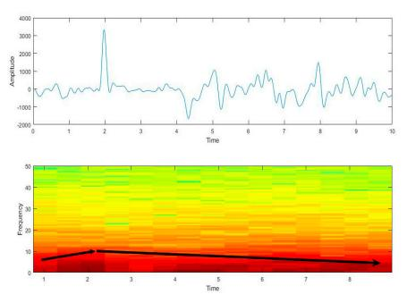
Figure 9. The time-frequency diagram of the airplane vibration signal.
