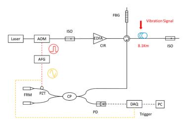
**Figure 1.** Setup of the  $\Phi$ -OTDR system.
