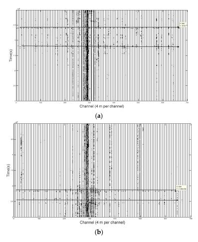
**Figure 6.** (a) Aircraft A vibration signal time delay in different locations of the optic fiber; (b) Aircraft B vibration signal time delay in different locations of the optic fiber.
