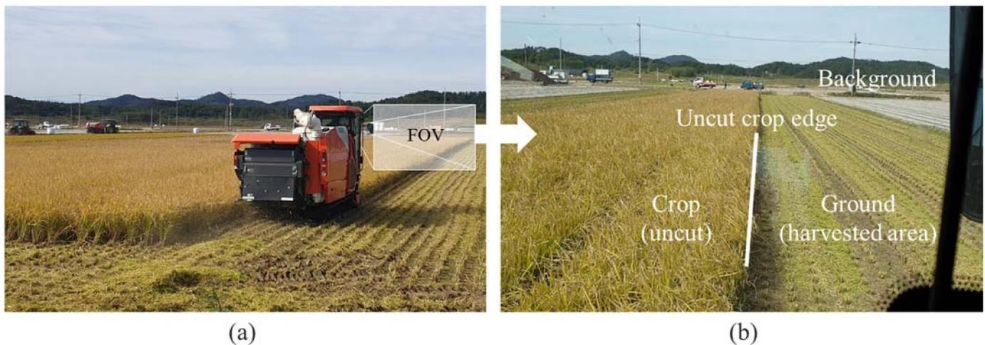
**Figure 1.** Harvesting scene of a combine harvester in a rice paddy (a) and a representative sample image including the operator's field of view (b).
