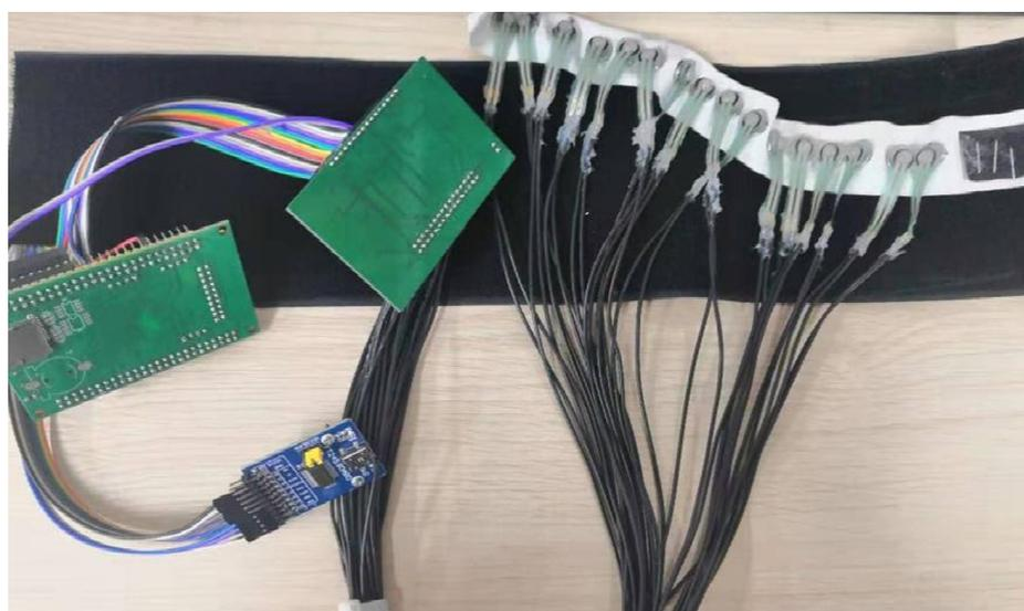
Figure 2. The hardware prototype for FMG acquisition.
