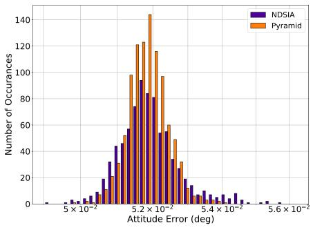
**Figure 5.** Test 4, Small OA Offset Perturbation, Attitude Estimation Error for Scenes with a Successful Star-ID.
