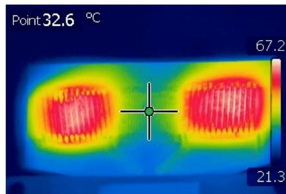
**Figure 6.** Temperature distribution of the sensor with 700 mA p-p excitation current at 100 kHz.
