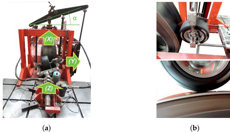
**Figure 1.** Test procedure applied to the intelligent tire: (a) The coordinate system used on the indoor tire test rig; (b) Instrumented tire set up on the tire test rig and its contact with the drum's surface.
