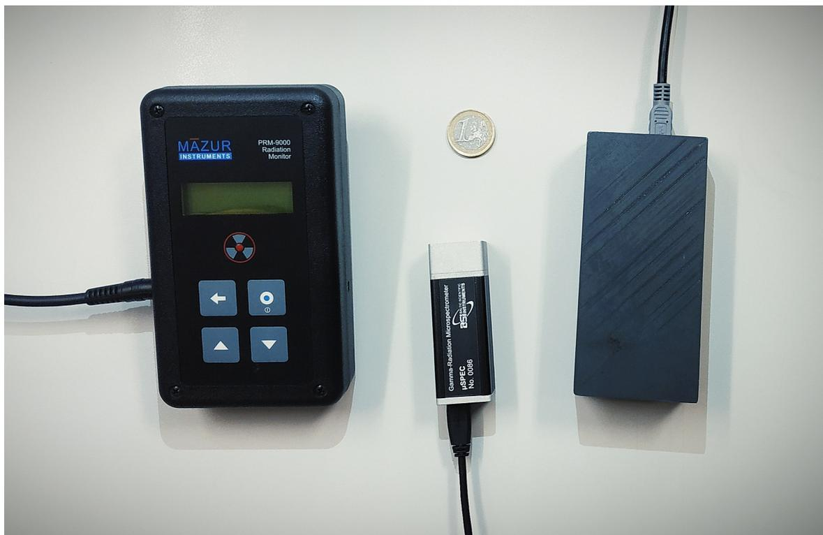
**Figure 2.** The radiological sensors used in this work. From left to right: the Mazur PRM-9000, the  $\mu$ SPEC 500 CZT, and the Sparkfun SEN-11345. A 1 euro coin is also present for scale.
